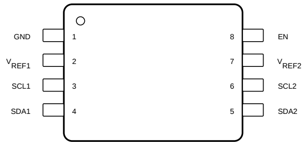
Figure 5-2. DCU Package 8-Pin VSSOP (Top View)
